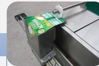
Pass carton through gluing wheel right to left
